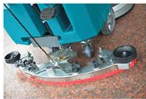
Integrated aluminum die casting water grill, anticorrosion
