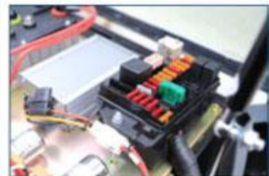
Electric control fuse
