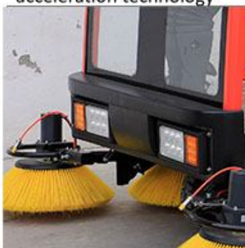
With water spray function, dust can be reduced
